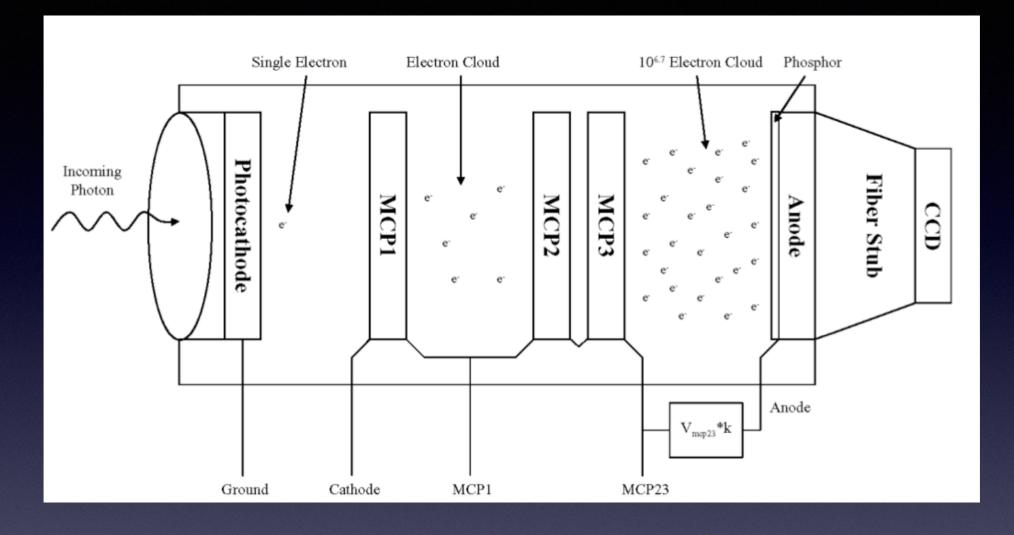
UVOT is a photon-counting instrument, doing on-board centroiding of photon splashes. This minimizes cosmic rays and dark count but creates coincidence loss (pileup) which makes counts non-linear and limits us to ~13th magnitude.\*
